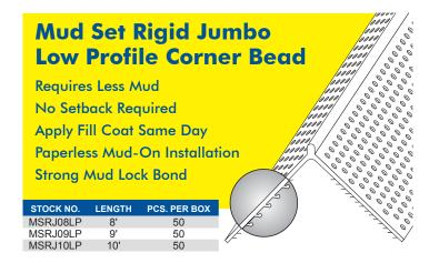
MUD SET BEADS ARE DESIGNED TO BE INSTALLED WITH HIGH QUALITY DRYWALL COMPOUNDS. DO NOT INSTALL WITH SPRAY ADHESIVES, STAPLES, NAILS OR SCREWS.
