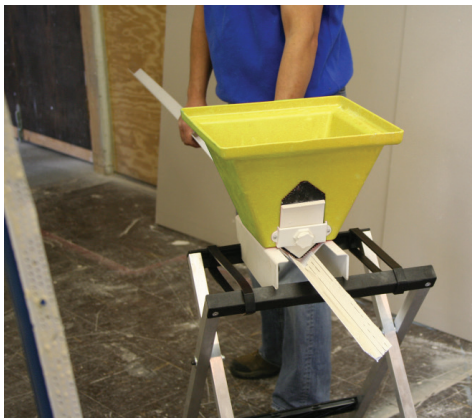
If using a compound tub apply mud/compound to drywall corner
