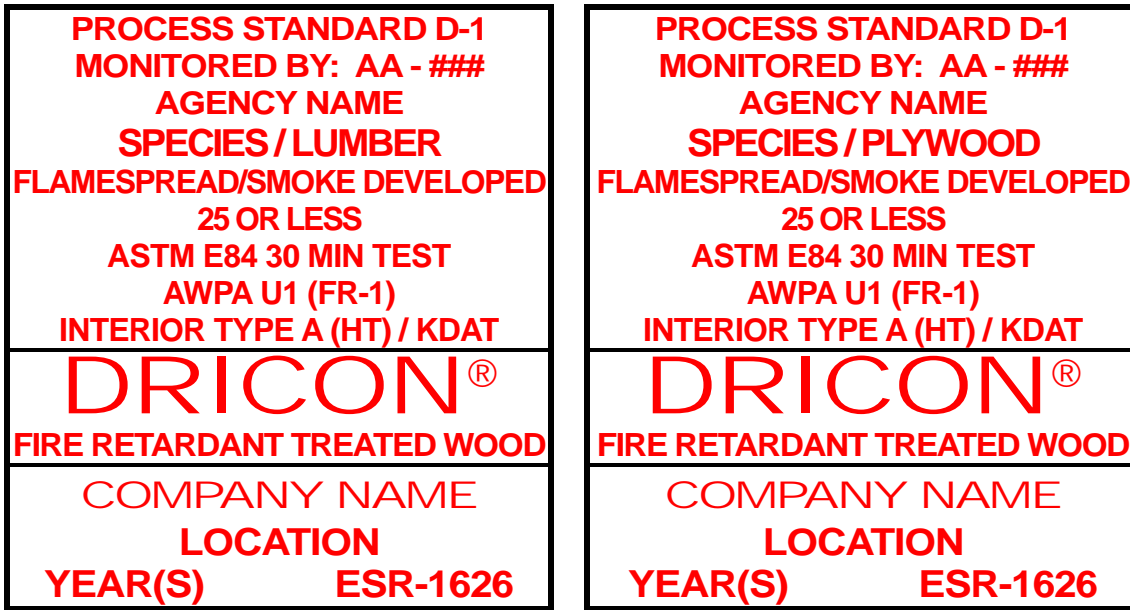
FIGURE 1—LUMBER AND PLYWOOD STAMPS 1,2,3
