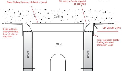
**Step 5.** Prior to the final sanding remove the tear away strip for a clean and crisp finish.
