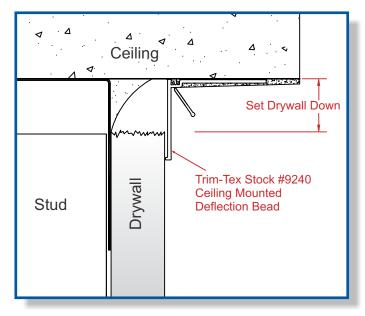
**Step 3.** Snip your bead to length and dry fit to the ceiling for accurate installation.
