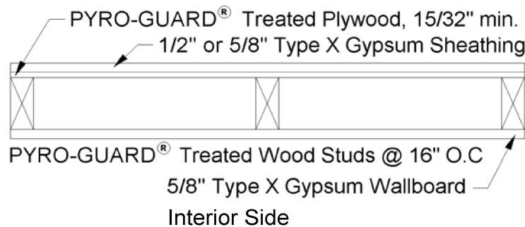
FIGURE 4—1-HOUR FIRE-RESISTANCE-RATED EXTERIOR WALL ASSEMBLY Use where wall is required to be fire-resistance-rated from the exterior and interior sides. (ESR-1791 1-HR)
