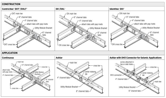
Note: All illustrations shown above are the 4 in. channel configuration. 6 in., 100 mm and 150 mm channel configurations can also be constructed.
