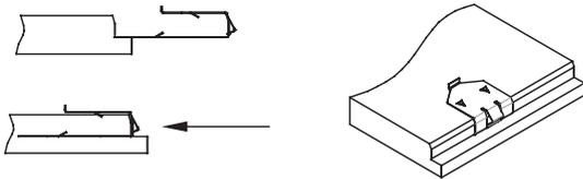
Once the A and B edges are engaged in the grid, gently push up on the "C" and "D" edges at the location of the Mid-Point Clip to engage the clip on the suspension system flange.
