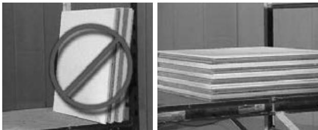
Do not stand the panels on edge. Keep them face-to-face, back-to-back and flat on the work surface.
