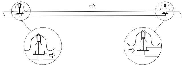
3. Lower the opposite edge out of the suspension system opening. Slide the panel off of the flange. Do not allow the panel to hinge or hang on the suspension system flange, as this may cause damage to the kerf, resulting in poor alignment when the panel is reinstalled.
