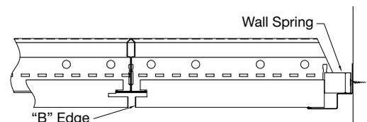
Wall Spring inserted between panel edge and molding
