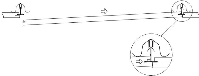
2. Raise the opposite "B" kerfed edge up into the suspension system opening.
