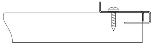
Insert the Vector Border Clip on the panel. Push an 8 x 9/16 sheet metal screw (or equivalent) through the clip into the plank to secure the border clip to the panel.
