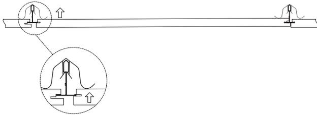
3. Slide the panel back onto the suspension system flange. Make sure that the "A" edge drops into position as shown.
