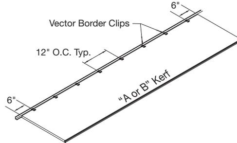
To install this panel, fully engage the "A" kerf on the suspension system. Raise the cut edge up until the border clips are above the wall molding. Slide the panel towards the wall until the access kerf of "A" edge drops down into the correct position. The Vector Border Clips will support the cut edge along the wall molding.
