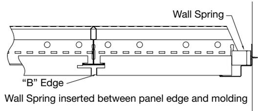
Wall Spring inserted between panel edge and molding
