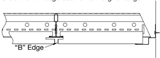
Use Mid-Point Clips on "C" or "D" edges (as detailed in section 2.3.1) if the border panel is greater than 30" wide.
