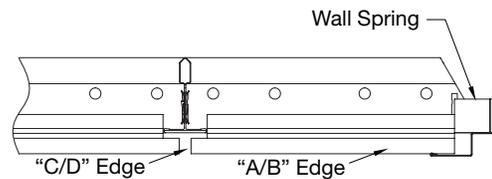
Wall Spring inserted between panel edge and molding
