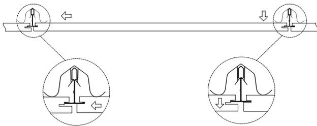
4. Required for panels over 30" in length. Gently push up on the "C" and "D" edges at the location of the Mid-Point Clip to engage the clip on the suspension system flange.
