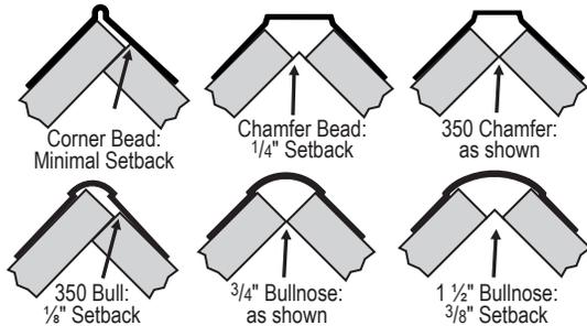
**Step 1:** Use minimal drywall setback on 90° Outside Corners & 350 Bull. For other bullnose and chamfer corners set the drywall back as shown to the left. Excessive setback will minimize bondability. Make sure the edges of the board are cleanly cut. Ripped or rolling paper will prevent the mud legs of the bead from sitting flat on the wall. Do not use the tapered edge of the board for outside corners.
